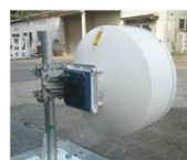
External Antenna Type WT with 60cm antenna
